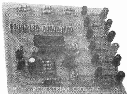
The circuit board of the pedestrian crossing: the cycle can easily be followed by watching the on-board LEDs. Note that the 4017 is upside down.
