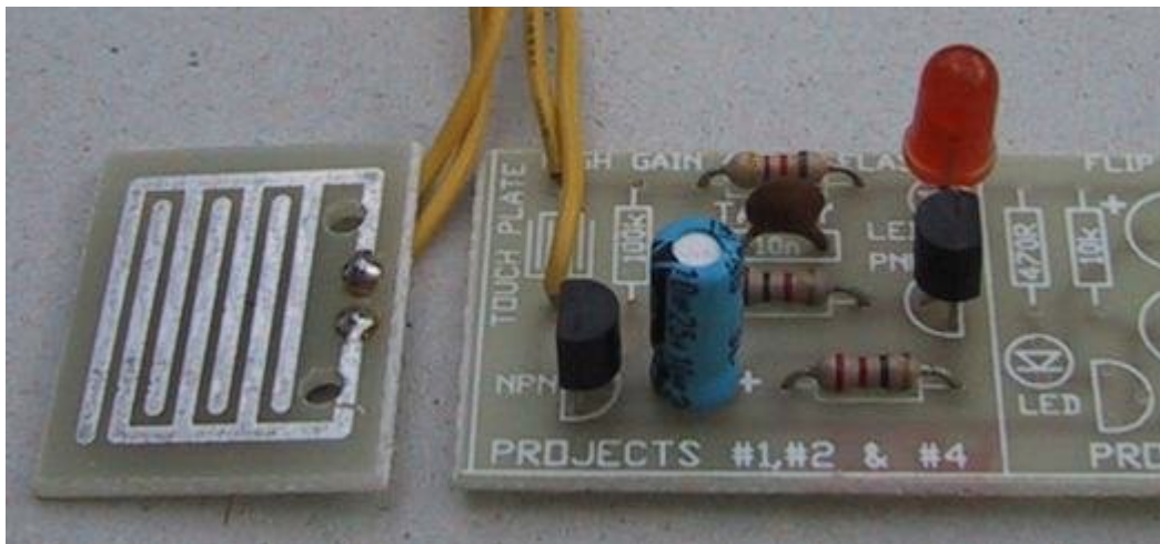
Project 2 with Touch Plate fitted to PC board
