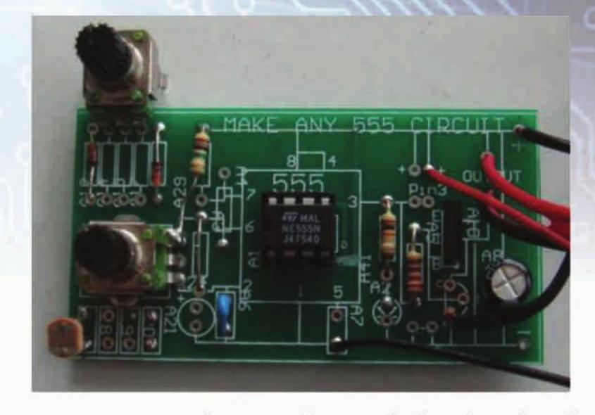
components and joining them with short lengths of wire or using the tracks already provided. Some of the tracks will need to be cut.
