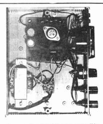
The upper voltage limit of the power supply will be set by the output voltage of the transformer and should not be above 15v for any of our circuits.
