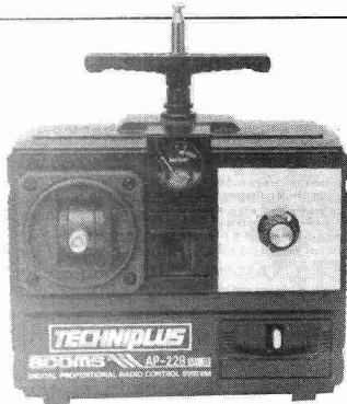
The modified transmitter. The crystal is visible below the control knob.
