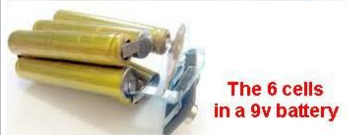
Fig 2. The CELLS in a 9v BATTERY
