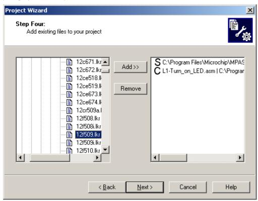
After you click "Next" and then "Finish" on the final Project Wizard window, you should be presented with an empty MPLAB workspace. You may need to select View → Project to see the project window, which shows your project and the files it comprises as a tree structure. For a small, simple project like this, the project window will show only two files: an assembler source file (.asm) and a linker script (.lkr).
