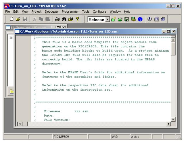
The MPLAB text editor is aware of PIC assembler (MPASM) syntax and will colour-code text, depending on whether it's a comment, assembler directive, PIC instruction, program label, etc. If you right-click in the editor window, you can set editor properties, such as auto-indent and line numbering, but you'll find that the defaults are quite usable to start with.
