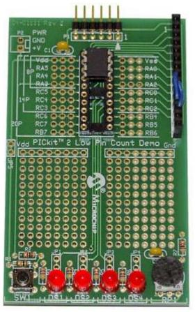
If you prefer not to solder components onto your demo board, you can use the LEDs on the board, labelled 'DS1' to 'DS4', by making connections on the 14-pin header on the right of the demo board, as illustrated on the left.
