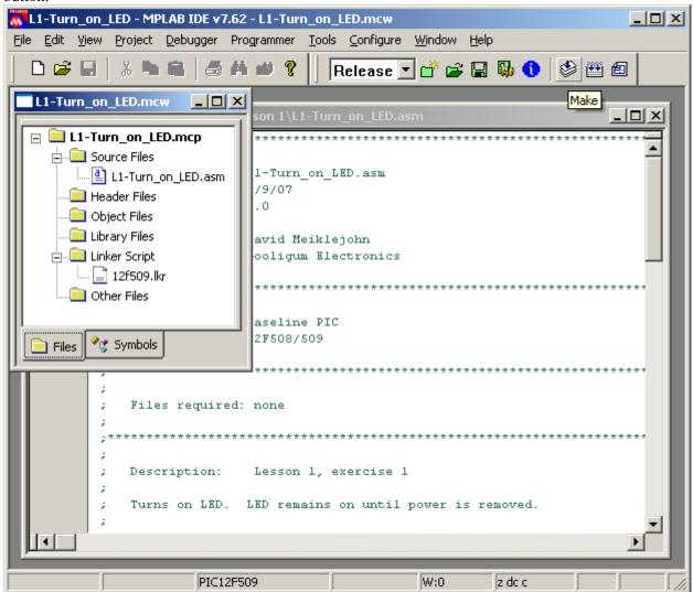
"Make" will assemble any source files which need assembling (i.e. ones which have changed since the last time the project was built), then link them together.
