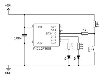
The instruction for placing the PIC into standby mode is 'sleep' - "enter **sleep** mode".
