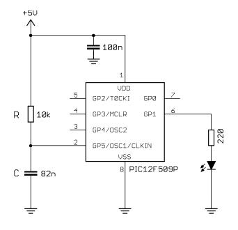
The voltage increases until it reaches a threshold, typically  $0.75 \times VDD$ . A transistor is then turned on, which quickly discharges the capacitor until the voltage falls to approx.  $0.25 \times VDD$ . The capacitor then begins charging through the resistor again, and the cycle repeats.
