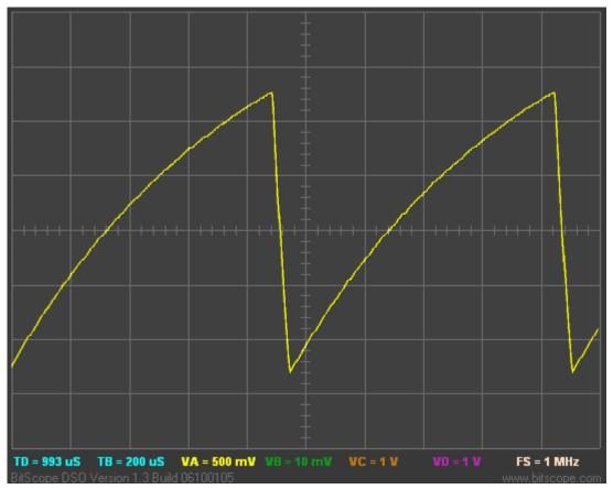
In theory, assuming upper and lower thresholds of  $0.75 \times VDD$  and  $0.25 \times VDD$ , the period of oscillation is equal to  $1.1 \times RC$  (in seconds, with R in Ohms and C in Farads).
