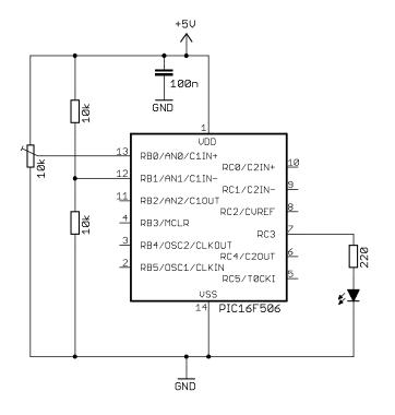
The 10 k $\Omega$  potentiometer on the demo board is already connected to C1IN+ (labelled 'RA0') on the board, via a 1 k $\Omega$  resistor (not shown in this diagram). But you must ensure that jumper JP5 is in place; it will be, if you haven't modified your demo board.
