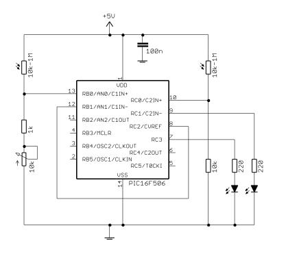
If you are using Microchip's Low Pin Count Demo Board, the connection from CVREF to C1IN- can be made by linking pins 8 and 12 on the 14-pin header.
