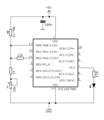
But before the comparator output can actually appear on the C1OUT pin, that pin has to be deselected as an analog input.
