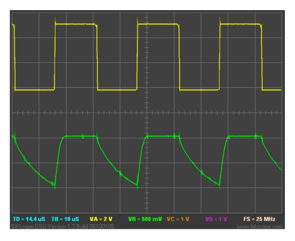
This degraded signal is not suitable for driving TOCKI directly; it doesn't go high enough to register as a digital "high". But it is quite suitable for passing through a comparator referenced to 0.6 V, so the internal reference voltage is a good choice here. Therefore the only comparator input needed is C1IN+, as shown in the circuit above.
