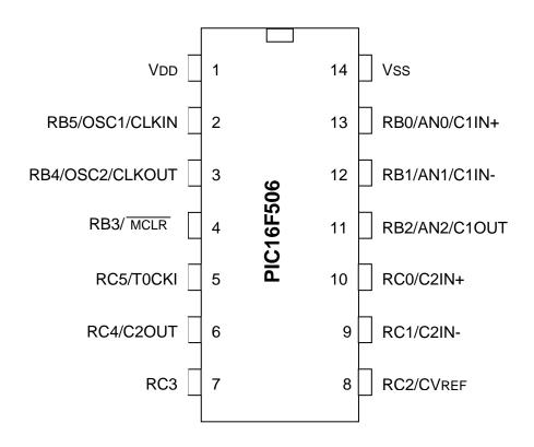
RC5 and T0CKI share the same pin, as was the case on the 16F505; to use RC5 as an output on the 16F506, you must first disable T0CKI by clearing the T0CS bit in the OPTION register.
