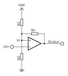
There are now two voltage thresholds: one (the higher) applying when the input signal is rising; the other (lower) applying when the input is falling. The comparator's output depends not only on its inputs, but on their history -a key characteristic of hysteresis.
